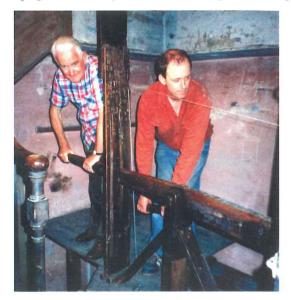
Fortunately, the original hand-pumping facilities have been retained on the Bermondsey instrument - almost all items recorded at Bermondsey on this CD had to be hand-pumped following failure of the electric blower. The manuals and pedals have separate reservoirs, thus requiring two people to pump.
